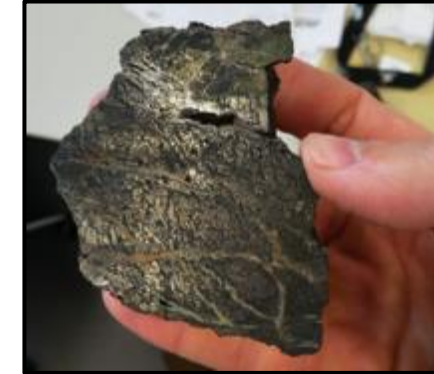
Massive Sulphide ore & thin-sections from Laxia-West, showing Chalcopyrite (Cp), Pyrrhotite (Po) and Cobaltite (Cb) from Patten, et al, 2022)
